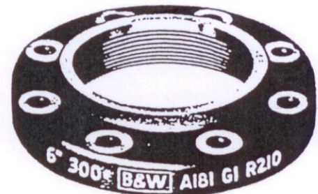
Figure 1-5. Threaded flange. (Courtesy of Hackney, Inc., a division of Trinity Industries.)
